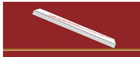
**Figure 2:** Hold the cleaving stone at ~30° angle with respect to the capillary tubing.
